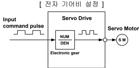
$$\text{전자기어비} \left( \frac{\text{분자}}{\text{분모}} \right) = \frac{\text{엔코더펄스수} \times 4}{\text{지령단위}} \times \text{감속비} \left( \frac{b}{a} \right)$$
